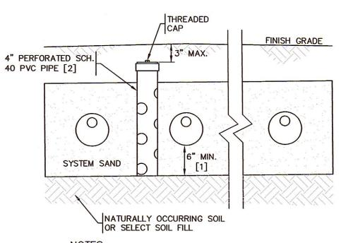
1] BOTTOM OF INSPECTION PORT TO BE INSTALLED FLUSH WITH BOTTOM OF SYSTEM SAND. [2] WRAP INSPECTION PORT WITH PERMEABLE GEOTEXTILE ABRIC TO ELIMINATE SAND INFILTRATION.
