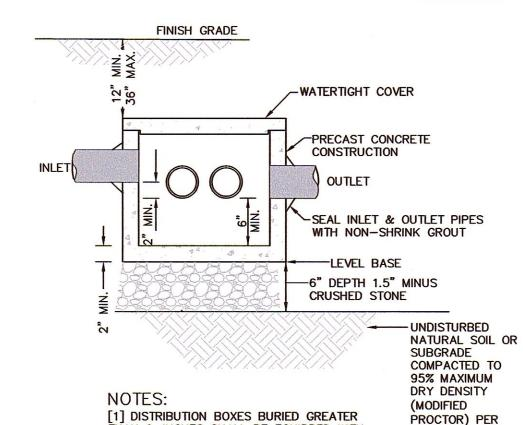
HAN 9-INCHES SHALL BE EQUIPPED WITH ASTM D1557. WATERTIGHT RISERS TO WITHIN 6-INCHES OF FINISH GRADE. 6-OUTLET DISTRIBUTION BOX
